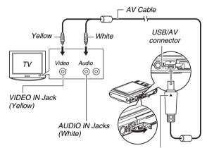
Making sure that the  $\nabla$  mark on the camera is aligned with the  $\triangle$  mark of the AV cable plug, connect the cable to the camera.
